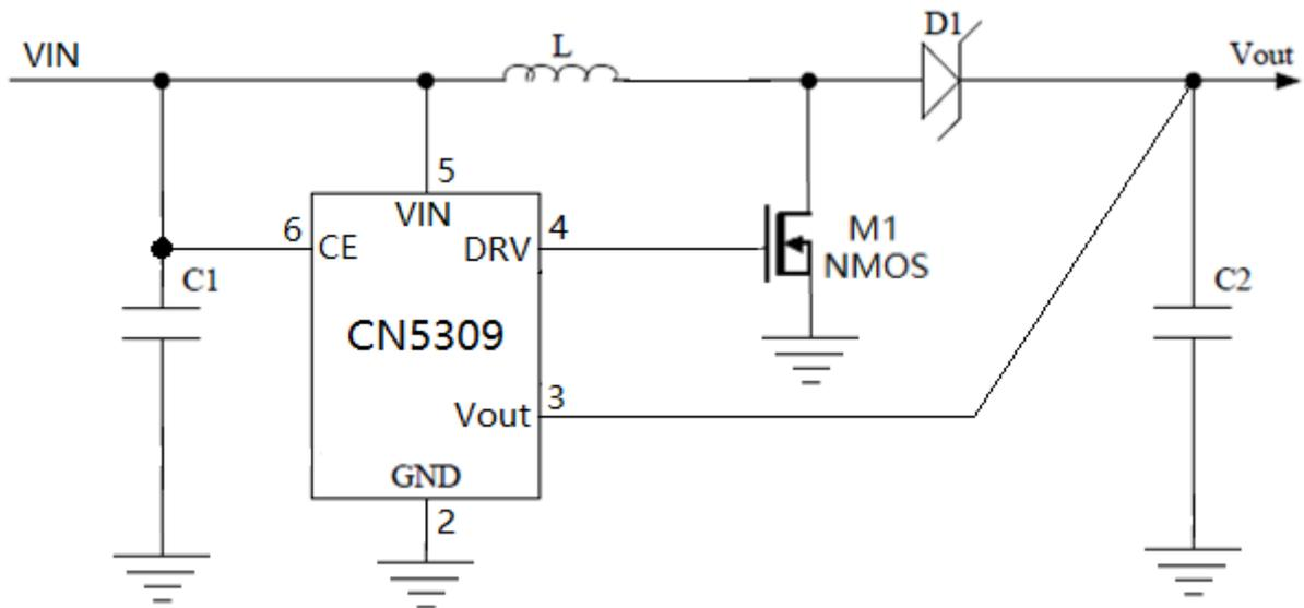
Figure 1 Typical Application Circuit (Fixed Output Voltage)
